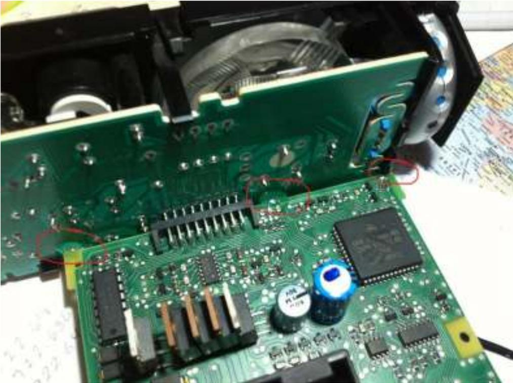
2. There's a small locating pin at the rear of the external housing that locates the circuit board. Fix - cut it off with a Stanley knife, as it pulls the rear circuit board away from the front board when you mount it in the housing. You could also apply some more epoxy here once you put it all back together.
