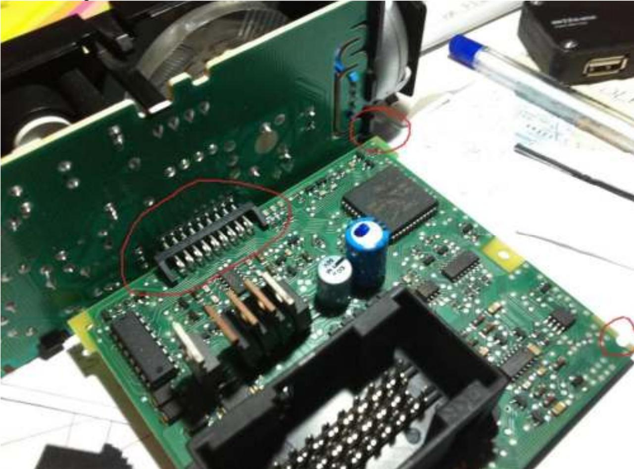
1. The front RHS of the rear circuit board hits part of the plastic surround of the front boardmounting, stopping it from fully pushing into the header socket. Fix - file some of the plastic away. Push the rear circuit board all the way into the header and apply some epoxy glue to hold it there.
