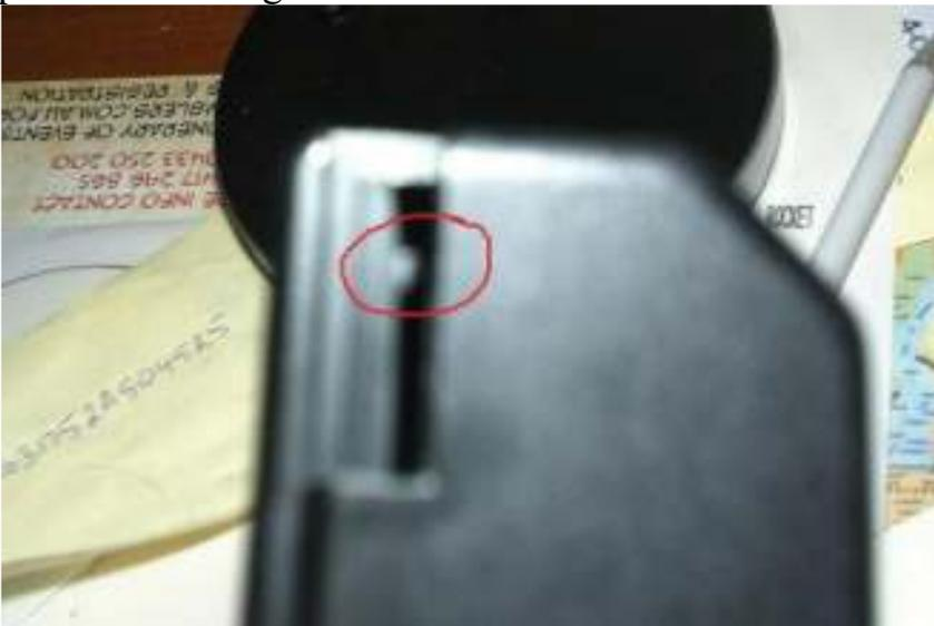
If you fix both the issues above you will get much better electrical contact between the front and rear circuit boards through the header and pins. I modified all three of my faulty units today, they now all work like new.
